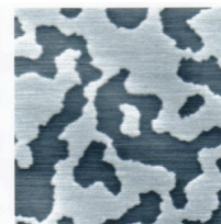
Fig. 2. Domain structure of Cu/8.5 nm Ni/Cu over a 12 micron square.
